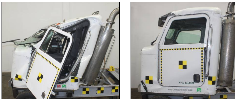
Fig. 12. Production and Reinforced Test Cab Comparison
