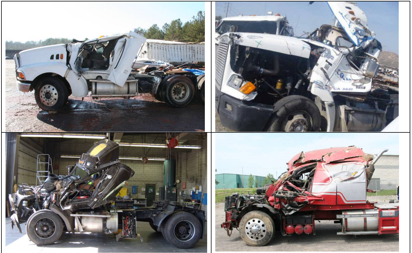
Fig. 8. Other Field Accidents with Similar Damage Patterns
