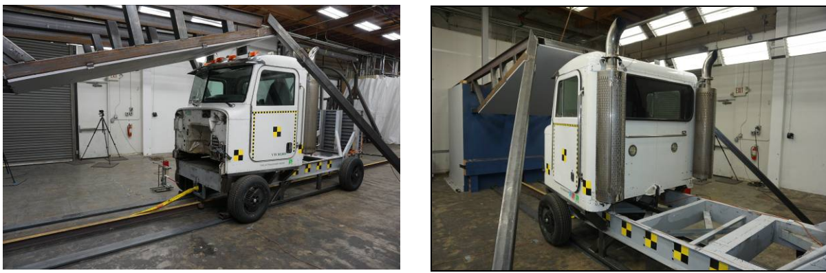
Fig. 9. Biaxial Sled Test Set-Up
