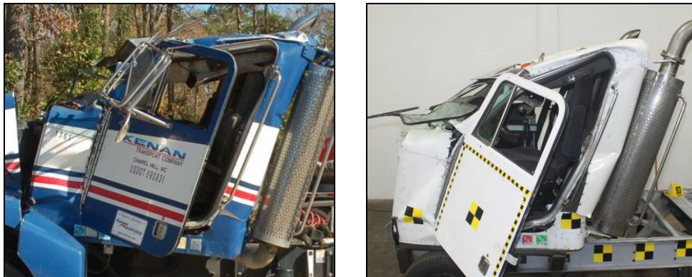
Fig. 11. Accident and Test Cab Comparison
